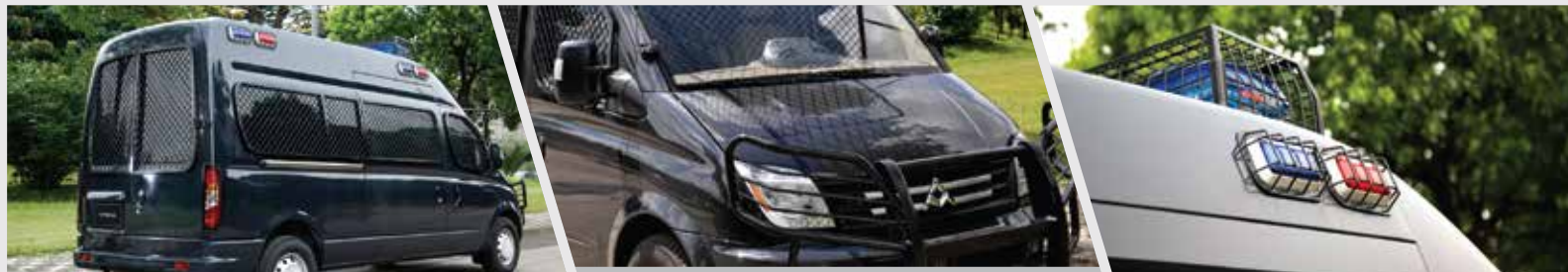
Headlights, alarm light, flashing lights with steel shield
