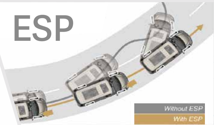
Latest generation of Bosch ESP9.1 electronic stabilization assistance system to provide full control on safety
