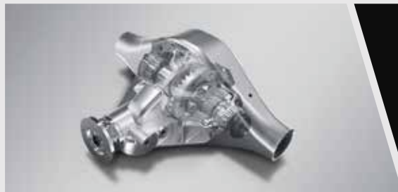
Rear Axle Differential Lock automatic locking is available when wheel speed difference reaches 100 rev/min, a must tough road conditions
