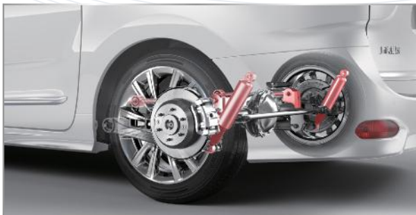
Nivomat fully automatic driving control system, combining comfort, trafficability and manipulation.
